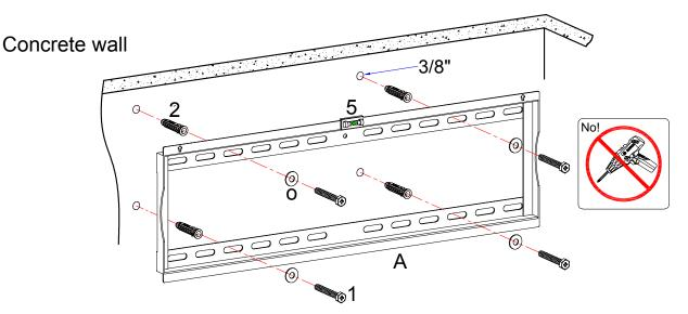
Figure 2 (keep the Wall plate level)
