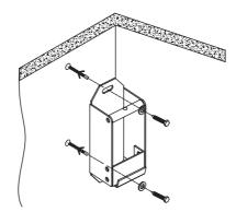
Figure 3 - Wood Stud/Concrete Mounting
