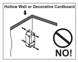
Figure 1 - Hollow Wall WARNING!
