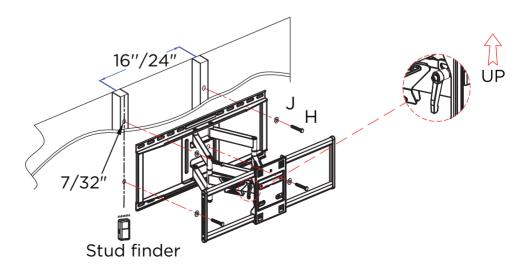
Figure 2 (keep the wall plate level)
