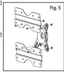
illustration (see Fig. 5). Use the M4 x 10 screws (C), spring washers (D), and M4 nuts (E) from the hardware kit.
