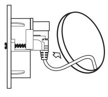
Level and screw Dog Ears until Housing is secure. Repeat at the bottom with the Male Housing.
