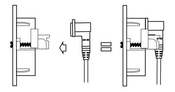
Snap on Female Crown over the Plug Tip and secure with screws. Repeat at the bottom with the Male Tip and Male Crown.
