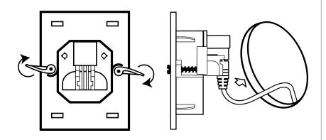
Level and screw Dog Ears until Housing is secure. Repeat at the bottom with the Male Housing.
